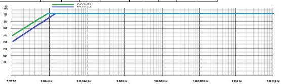
\* FCP-22 AND 23 SERIES 100dB from 14KHz TO 10GHz measured in a 50 Ω system per MIL-STD 220A load condition
